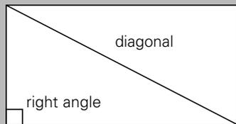
This means that the diagonal of a rectangle is always longer than either of the sides. As a result, rectangular covers can always be dropped through their corresponding holes if the lips are small. Because a square is a rectangle, the same reasoning applies to squares.
